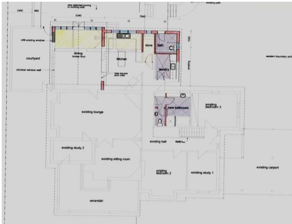
Figure 8.0, Ground Floor Plan, Wayne McPhee and Associates Pty Ltd in 1997 for Frances and Sean Foster. The changes to central bathroom were not executed as per the drawings, creating one large bathroom without separate WC.
